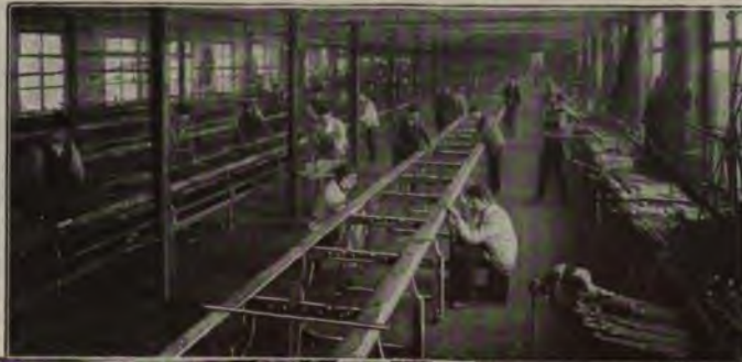
Room of the same factory where these castings are being put together so as to form the frame of a machine for spinning cotton thread, such as is shown on page 56.
